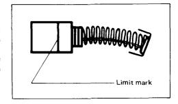
Use a screwdriver to remove the brush holder caps. Take out the worn carbon brushes, insert the new ones and secure the brush holder caps.
